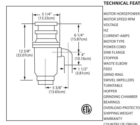
VOLTAGE 110 - 120 ΗZ 60 **CURRENT-AMPS** MOTOR TYPE Permanent Magnet **POWER CORD** Attached SINK FLANGE Stainless Steel STOPPER Positive Seal **WASTE ELBOW** ABS FEED Continuous GRIND RING Carbon Steel SWIVEL IMPELLERS Stainless Steel **TURNTABLE** Carbon Steel **HOPPER** Polycarbonate 940 **GRINDING CHAMBER** Corrosion Proof Glass Filled Polyester **BEARINGS** Permanently Lubricated; Sleeve Type OVERLOAD PROTECTOR
